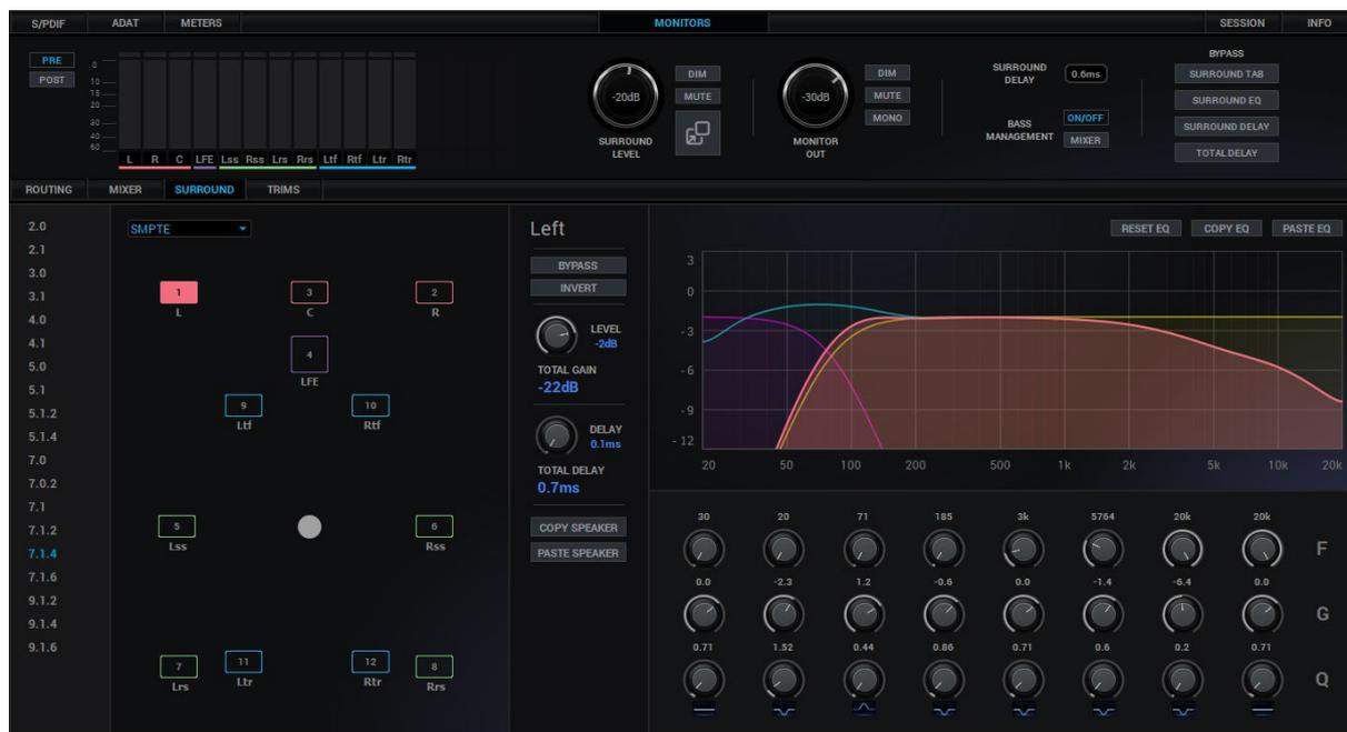
The Antelope Audio Surround / Immersive Monitoring System provides monitoring control functionality and speaker calibration processing for up to 16 channels of surround or immersive audio. Formats from stereo up to 9.1.6 Dolby Atmos are supported while maintaining customizability within the 16-channel limit for any unorthodox setup requirements.
