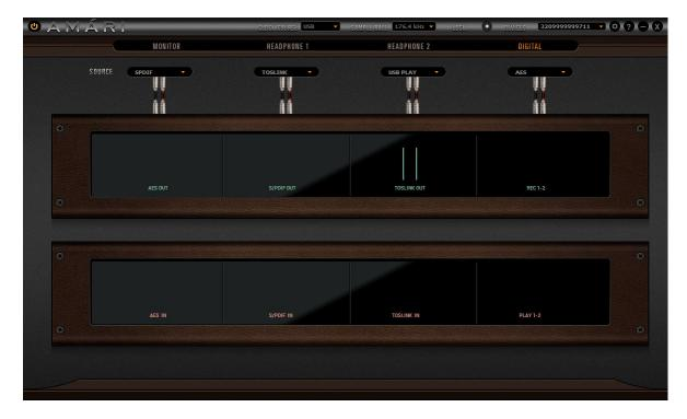
This section manages signal routing for the digital inputs and outputs. The audio source for each output can be chosen freely from the drop-down menus. Input and Output level meters are found here as well.
