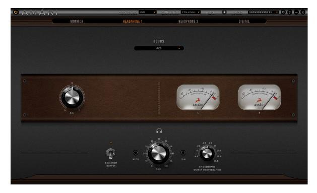
These sections control the Headphone 1 & Headphone 2 outputs of the AMÁRI. They feature identical functionality, except for the balanced output switch and impedance adjustment knob.
