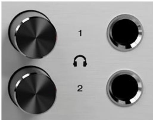
Headphone outputs H1 - H2 with gain adjustment knobs
