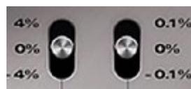
Adjusts the Word Clock sample rate to sync to PAL/NTSC video.
