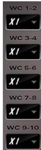
5 dropdown menus used to multiply or divide the current selected sample rate on pairs of 2 Word Clock outputs. This way, the OCX HD can output up to 5 different sample rates on each pair of 2 Word Clock outs. That is, if the sample rate is 96kHz, dividing it by two makes 48kHz and multiplying it by for 4 makes 384kHz.
