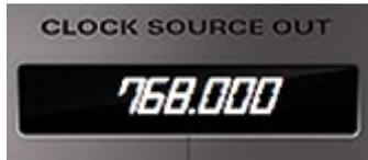
Indicates the output sample rate. This might change if the sample rate is affected by pull ups / pull downs.
